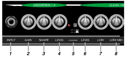
1. INPUT: Use this 1/4" jack to connect your bass to the amplifier by means of a shielded instrument cable.
